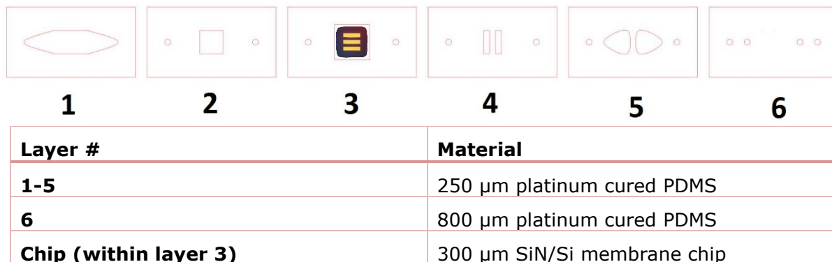
Figure 2. Gasket stack order of assembly
